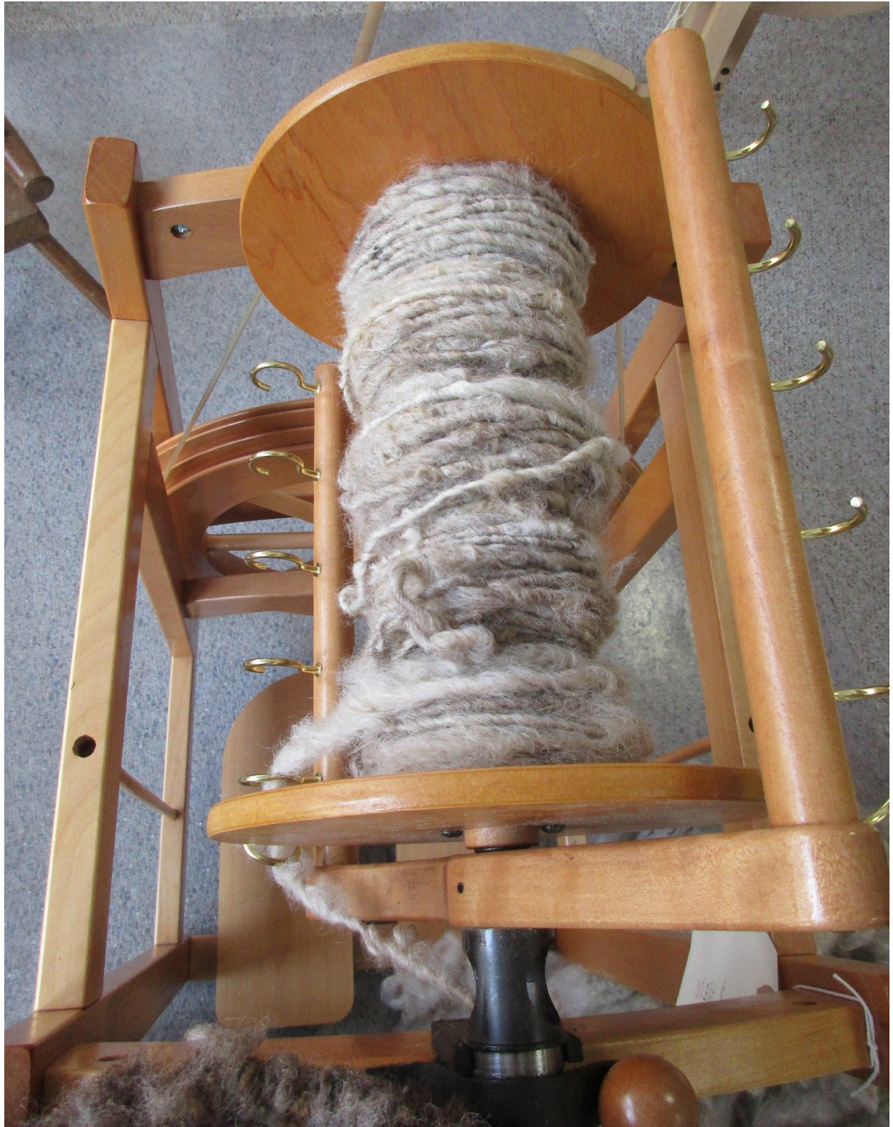
Yarn winding on the bobbin of the Country Spinner 2.
